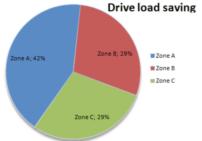
Figure 12. The percentage of total forming section drive in each zone
