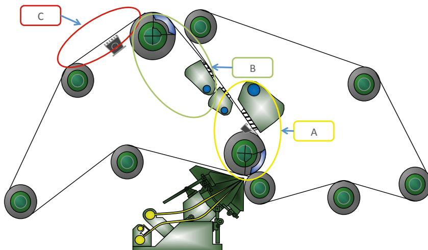
**Figure 5.** A side elevation drawing of the forming section. To simplify analysis the section has been divided into 3 zones.
