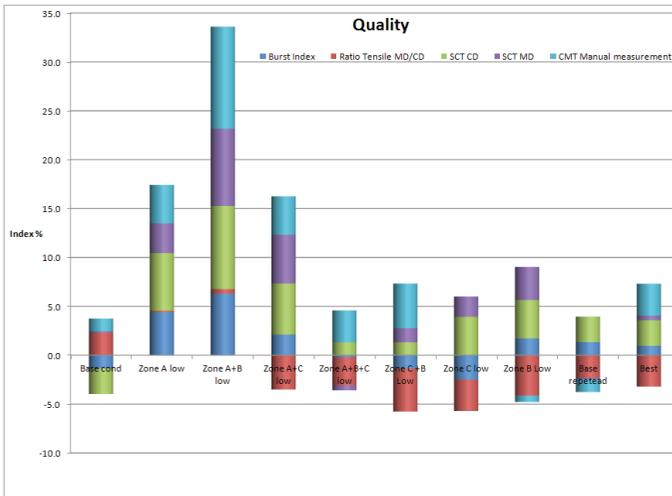
Figure 11. The “Quality Index” is compiled by summing the percentage change in properties from the standard settings
